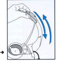
Note: for the helmets equipped with a visor return system: press the two buttons at the top of the visor simultaneously in order to unlock it. Six lower locking positions can be used.
